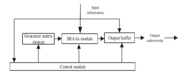
Figure 1: construction of the LDPC coding based by Chinese Digital Radio.
