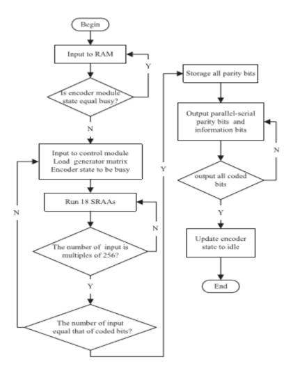
Figure 2. The controlled algorithm about to rate LDPC encoder system.
