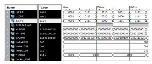
Figure 5: variable node function simulation results
