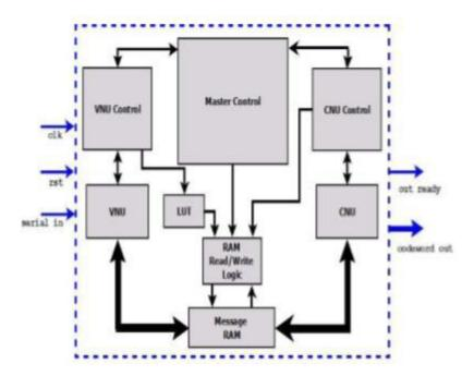
Figure 3: LDPC decoder architecture.
