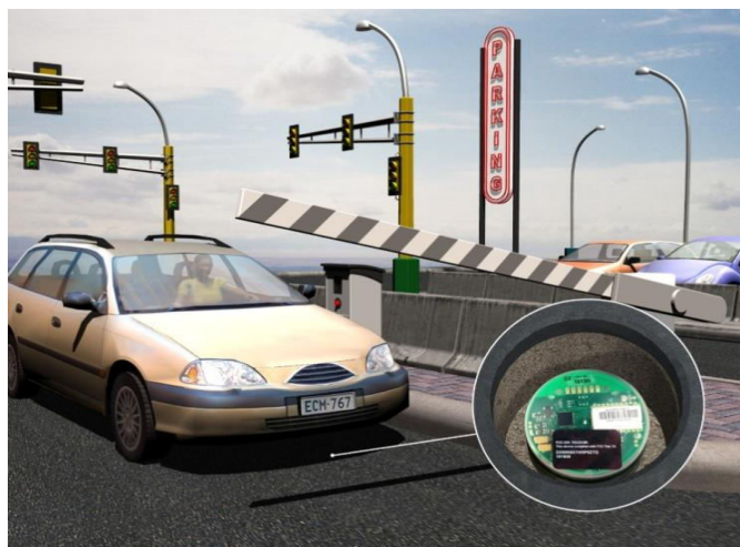
Fig 4 Wireless Magnetometer detects vehicle near an automated gate
