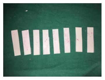
FIG 7-Prescale Fujifilm showing colour changes after biting.
