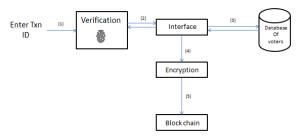
Fig 3: Voting Module Flow Diagram
