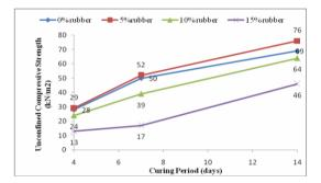
Figure 2: Variation of Unconfined Compression Test Results with 2% Cement and Different % of ragged Rubber at Different Curing Periods
