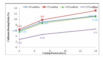
**Figure 5:** Variation of California Bearing Ratio Unsoaked Test Results with 4% Cement and Different % of
