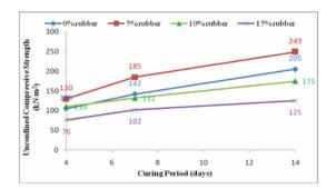
Figure 3: Variation of Unconfined Compression Test Results with 4% Cement and Different % of Shredded Rubber at Different Curing Periods
