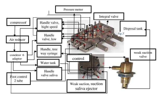
Figure 7 The wind source from the compressor to a handpiece, tree way syringe, and weak suction saliva ejector.
