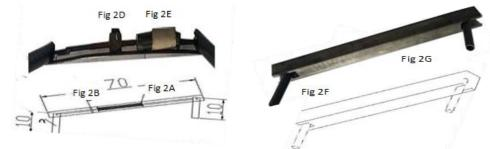
Figure 2 Operator lamp arms and instrument table arms, Length of the instrument table arms(70cm) and operator lamp arms(80cm), shock breaker spring(2A, 2E); limiting spring(2B); vertical round iron 10 cm(2C, 2F); retainer(2D).
