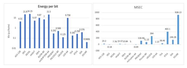
Figure 4: Energy Consumption of different algorithmsFigure 4: MSEC value of different algorithms
