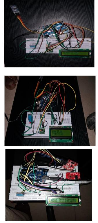
Figure.5. Snapshots of results using LM 35, BPM using MAX30105 and DHT11 Sensor in slave circuit.
