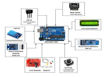
Figure.1.Architecture of Slave Circuit
