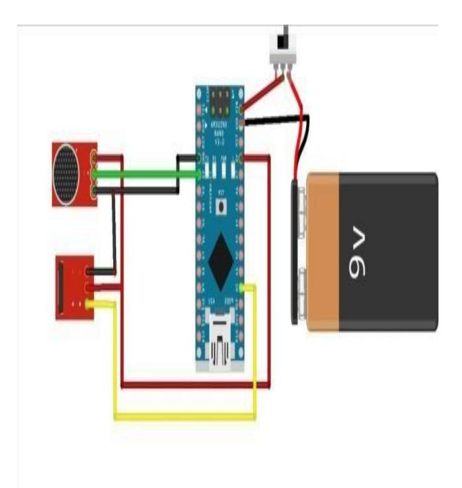
Fig.6 Basic Circuit Diagram of IR Sensor
