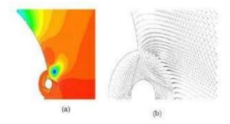
**Fig.17** The static pressure contour of the axial vane(a) –formation the vortex above the axial vane and stream lines(b)
