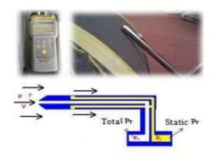
Fig.8 Digital manometer and pitot tube.
