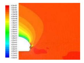
**Fig.16** Static pressure contour of the UAV with mounted vane.
