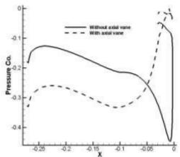
Fig.18 The pressure coefficient distribution on the body of the UAV in both cases, without and with axial
