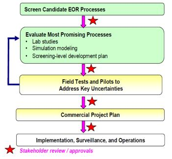
Figure 1. EOR Evaluation Workflow (after Selamat et al., 2008)
