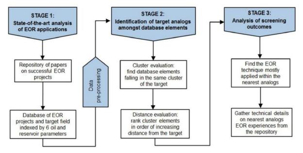
Figure 3. Detailed Workflow of ER Screening Procedure (after Siena et al., 2015)
