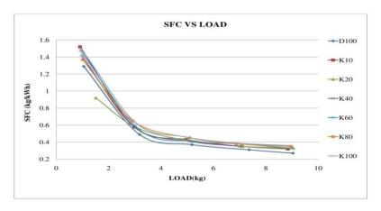
Fig. 3: Variations of Specific fuel consumption with Load
