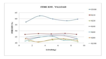
Fig. 4: Variations of Indicated thermal efficiency with Load
