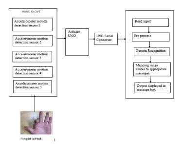
Fig.2 Block Diagram of the proposed system
