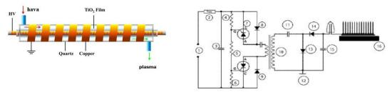
Fig. 1. Schematic of the nano- plasma air purification device.
