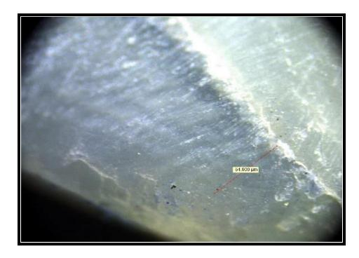
Figure 6: Dye penetration in Conventional group
