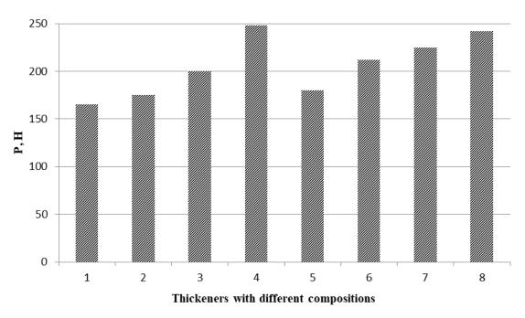
Figure 1. Mechanical strength of printed cotton fabric with different thickener compositions:
