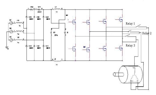
Fig. 8 open circuit fault in z source inverter fed induction motor
