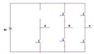
Fig. 3 Proportional circuit when open circuit deficiency happened.
