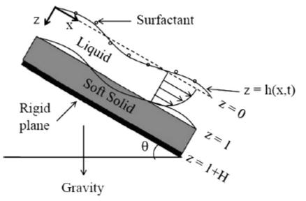
Fig. 1. Schematic of the configuration considered in the present work: Surfactantladen Newtonian liquid film falling down an inclined plane coated with a soft, deformable neo-Hookean solid layer.
