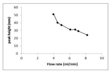
Fig (6) Effect of flow rate on peak height
