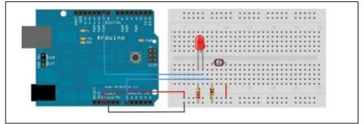
Fig (3) the electronic components of fluorimeter device
