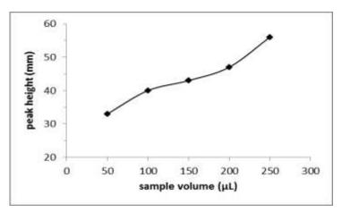
Fig (7) Effect of sample volume on peak height
