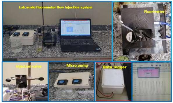
Fig (1) Lab-made fluorimetricflow injection system
