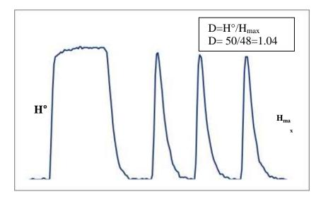
Fig (10) Dispersion cofficient in fluorometer FIA system
