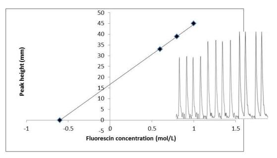
Fig. (11)0.6 mol/L fluorescein by standard additions method
