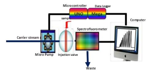
Fig (5) A singlemanifold for fluorescein determination by the lab-buildfluorometeric-FIA
