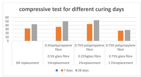
Graph: Compressive test for different curing ages
