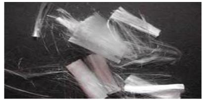
**Figure:** Polypropylene fibre
