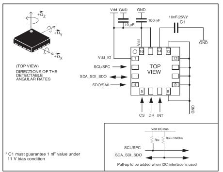
Fig.7 L3GD20 electrical connections and external components
