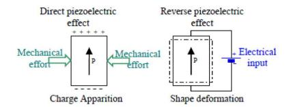
Fig.1 Electromechanical transfer by piezoelectricity
