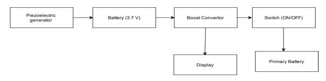
Fig.10 Block diagram for Piezoelectric generator
