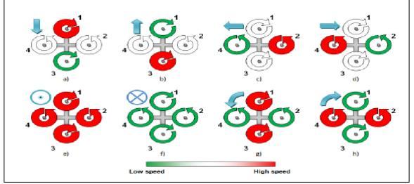
Fig.4 various movements of quadcopter
