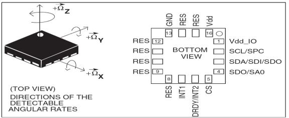
Fig.6 Pin connection of L3GD20
