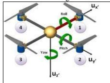
Fig.3 Common degrees of freedom of quadcopter
