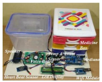
Figure 3 Prototype Model of Proposed Smart healthcare System
