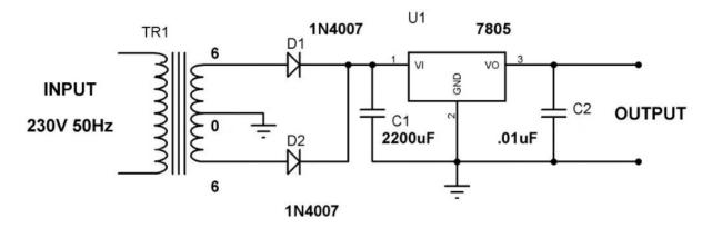
Figure 1. Power supply circuit
