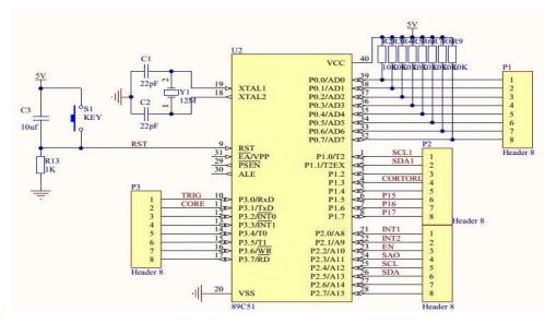
Figure3. Circuit schematics of AT89c51
