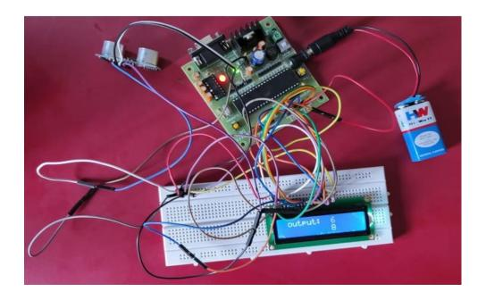
Figure6. Ultrasonic sensor interfacing with 89c51
