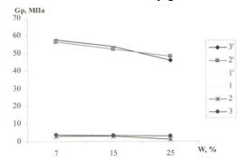
Fig-2: Dependences of the change in the ultimate strength of the soybean husk on its moisture content when breaking along the major axis (4, 5 and 6) and along the minor axis (4, 5 and 6) 4 and 4. Krasnodarskiy cultivar grown on irrigated lands, 5 and 5 grade Tashkent, grown on irrigated lands: 6 and 6 grade Russian grown on irrigated lands.
