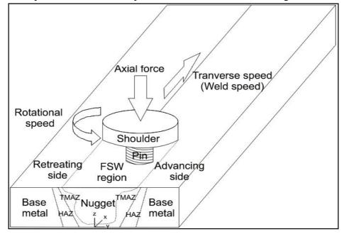
Figure 2.1 Friction stir welding process (Nourani 2011)
