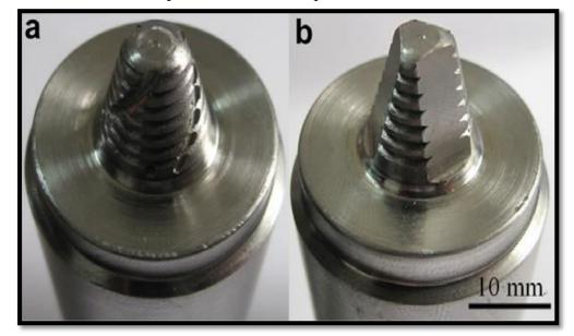
Figure 2.3 FSW tool pin profiles: (a) Threaded and tapered with three spiral flutes and
