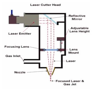
Figure .5. Laser cutting technology
