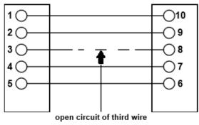
Fig 2.Open Circuit
