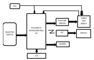
Fig 1. Proposed System Block Diagram
