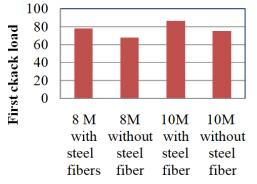
Mix Id Cracking Loads
