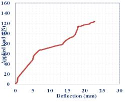
Load vs. deflection curve without steel fibers10
