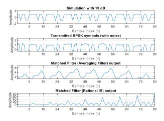
Fig-5: Simulation waveform for BPSK data transmission
