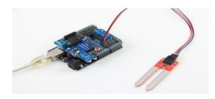
Figure 3: Soil Moisture sensor
