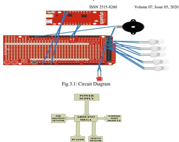
Fig: 3.2 Line diagram for home automation
