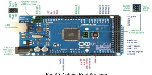
Fig: 3.3 Arduino Bord Structure
