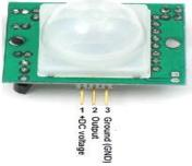
Fig.4.1: PIR motion sensor
