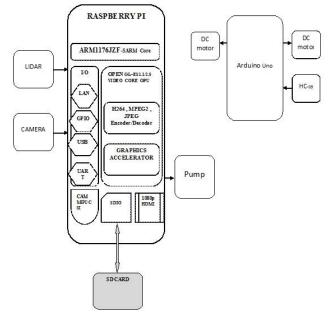
Fig. 1.Block diagram of the Robot
