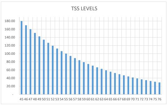
From the TSS estimation graph data above, it can be seen that the estimated time for waste treatment with a floating septic tank requires a residence time of 76 days until the effluent time with the resulting TSS parameters is in accordance with raw quality standards or is safe for disposal to the surrounding environment.
