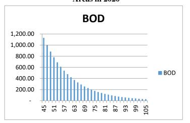
Based on the BOD graph data, it can be seen that the estimated time for the results of floating septic tank waste treatment requires a residence time of 105 days until the eluent time with the resulting BOD parameters align with the quality standards. From the graph, it can be concluded that the longer the residence time of BOD, the lower the level.
