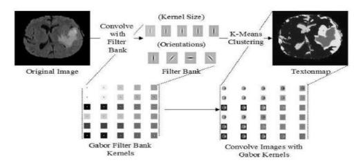
Fig. 1. Construction of the orientation image using Gabor filter bank.
