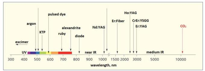
Figure: 1. Lasers used in medical practice, their radiation wavelengths.
