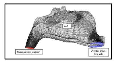
Figure 3- Volume mesh of 3D computational model of human nasal cavity (13)
