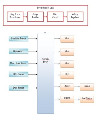
Fig. 2 Block diagram of the transmitter unit
