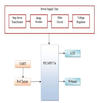
Fig. 3 Block diagram of the receiver unit
