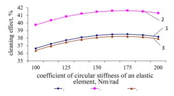
Figure.7. Change of the cleaning effect from changing the coefficient of circular stiffness of the elastic roller element
