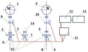
Figure. 2,a. Electric strain gauge circuit
