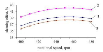
Figure.5. Graphs of changes in the cleaning effect depending on the frequency of rotation of the peg drum
