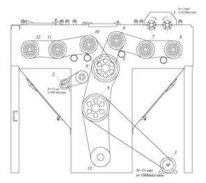
Figure.1. Kinematic diagram of the cotton ginner drive with a new drive layout A feature of the proposed drive scheme of the unit is the kinematic connection between the main working bodies: saw cylinders 4,5 pegs 7,8,11,12 and brush drums 6,7 waste augers 13. This ensures the work of the working bodies interconnected, as a single flow chain. This allows a decrease in slaughtering, an increase in the cleaning effect, and a decrease in fiber and seed damage.
