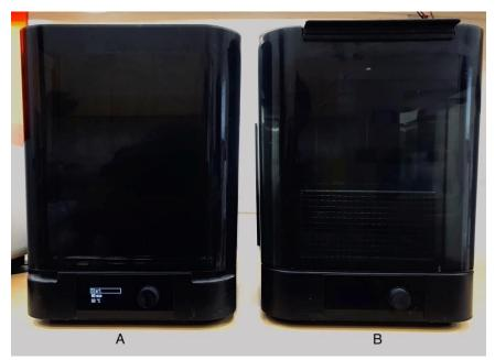
Figure 2 A: UV curing unit
