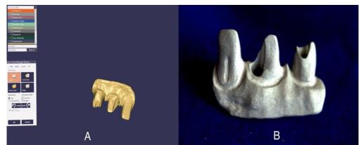
Figure 3 and B: 3D design and metal printing (implant restoration framework)
