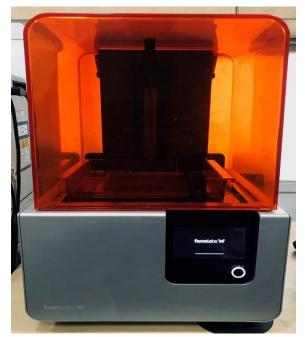
Figure 1: SLA 3D PRINTER (FORM2 FORMLAB)
